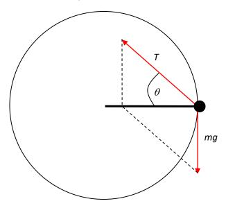
(ii)  $T\sin\theta = mg$  and  $T\cos\theta = \frac{mv^2}{R}$ . I.e. the resultant force is  $\frac{mv^2}{R}$  along the rod. Since the tension is the hypotenuse of a right-angled triangle:
